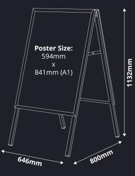
Overall Dimensions: 646mm(w) x 800mm(d) x 1132mm(h) External Frame Size: 625mm x 872mm Poster Size: 594mm x 841mm (A1) Visible Poster Size: 576mm x 824mm Weight: 5.3kg Packaged Weight: 7kg
