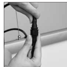
Fix the power source to the short side of the LED box frame's jack
