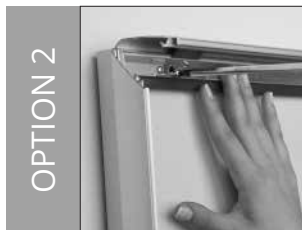
Open the PVC Panel of the Smart LED box outwards. Fix on the wall by using the mounting holes under the PVC profiles with the help of screws and wall plugs
