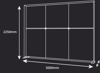
Weight: 28kg Extrusion: 120mm
