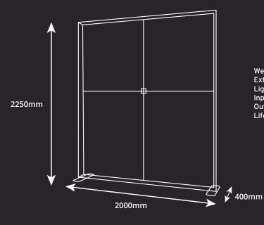
Weight: 24kg Extrusion: 120mm Lights: Lumen 260 per Bulb / 6500K Kelvin / Daylight Colour Temperature Input Power: 100- 240V 50/60Hz Output Power: 24V 6.35A Life Expectancy: 50,000 Hours
