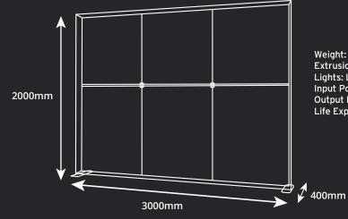
Weight: 28kg Extrusion: 120mm
