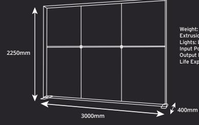
Weight: 28kg Extrusion: 120mm
