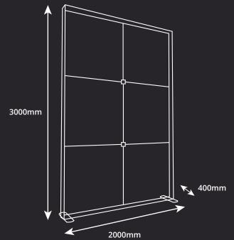
Weight: 28.6kg Extrusion: 120mm
