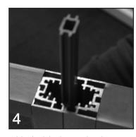
Slide inline link in between the side trims as shown to link the screens.
