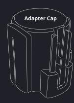
Adapter Caps come in two sizes, **64mm** or **70mm**. Each has an allowance for 1mm either side.
