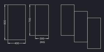
Tile construction is from 6/9mm medium density fibreboard (MDF) adhered (using water based adhesive) to 18mm sound absorbing foam.
