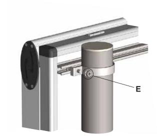
Lastly, screw the nuts (E) onto the bracket bolts (D), tightening with a spanner.
