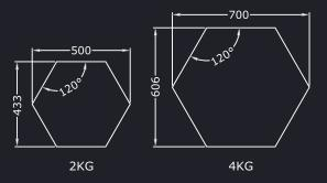
Tile construction is from 6/9mm medium density fibreboard (MDF) adhered (using water based adhesive) to 18mm sound absorbing foam.
