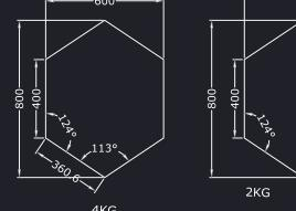
Tile construction is from 6/9mm medium density fibreboard (MDF) adhered (using water based adhesive) to 18mm sound absorbing foam.
